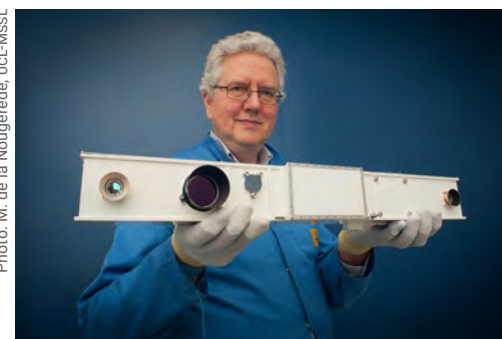
The image shows Andrew holding the Engineering Model of the Rosalind Franklin PanCam instrument, which we hope will look for past life on Mars later in the 2020s.
